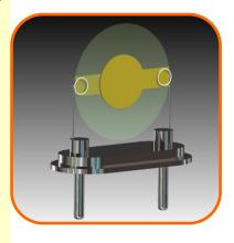
This high quality 10MHz polished quartz crystal has gold plated electrodes and it is installed on a socket suitable to be used with all the Eureka chambers for liquids. It is possible to make measurements in gaseous phase installing only this quartz in the Eureka oscillator base or using a suitable chamber for gas.
