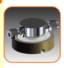
This is a flow-through measurement chamber for gases, the chamber is made of AISI316 Stainless Steel, the inlet and outlet connectors are 1/4" Swagelok<sup>TM</sup>, it works with the quartz crystal at 20MHz code 010868-07 or 010868-08.
